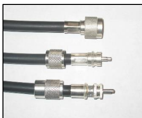
PL-259 crimped on RG8 coax. Center pin requires soldering.
