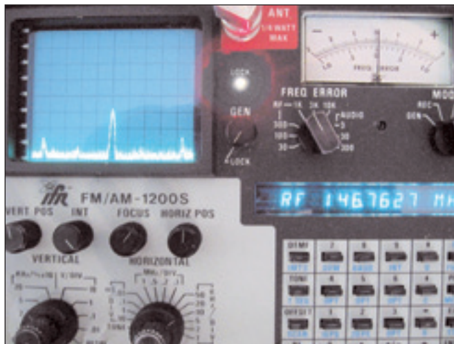
Figure 1 — The offending signal at 146.7627 MHz 30 dB above the noise.
